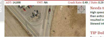
Needs to be Addressed High speeds on SR 74 produced smaller than anticipated gaps. High speed crashes resulted in severe and fatal injuries. Skewed intersection reduces sight distance.
